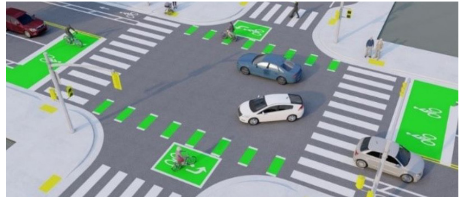
Green-Colored Transition Striping, Source: VDOT
