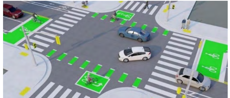
Green-Colored Transition Striping, Source: VDOT
