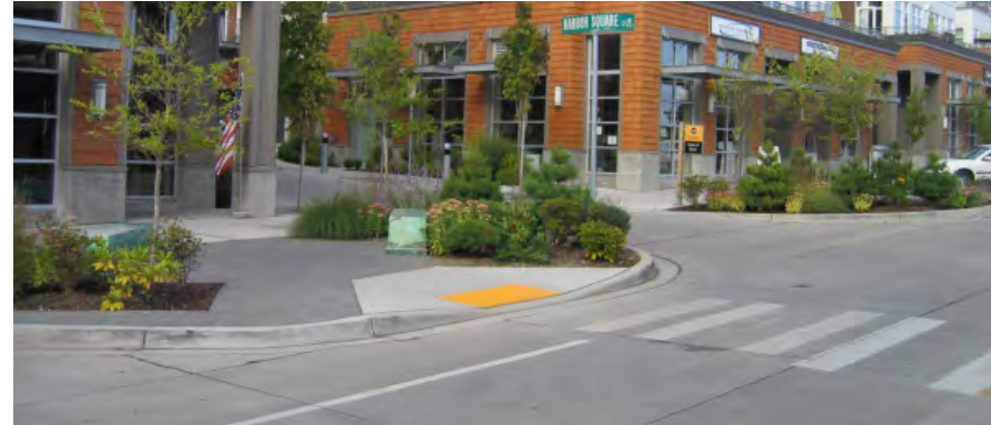
Bulb Out / Curb Extensions
