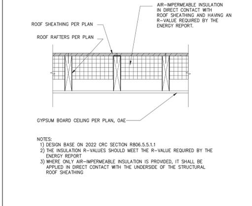
12 INSULATION @ UNVENTED ROOF ASSEMBLY IMPERMEABLE ONLY SCALE: 1"=1'-0"
