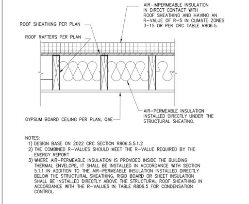
4 INSULATION AT UNVENTED ROOF ASSEMBLY-OVER/UNDER SCALE: 1"=1'-0"
