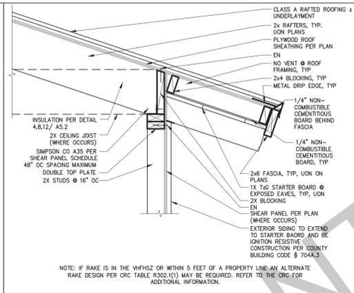
5 IGNITION RESISTIVE EXPOSED RAFTER EAVE SCALE: 1"=1'-0"
