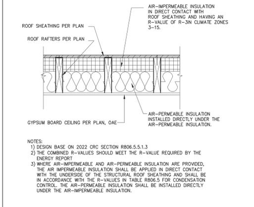
8 INSULATION @ UNVENTED ROOF ASSEMBLY BOTH TYPES SCALE: 1"=1'-0"
