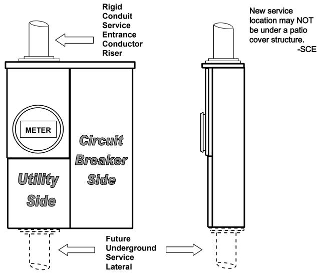
A surface-mounted combination service rquires no raceway provision for future underground feed. When new service is semi-flush or flush mounted, a 3 inch rigid raceway is needed. Cap straight stubout at a depth of 12 inches below grade. A sweep is capped at 30 inches below grade.
