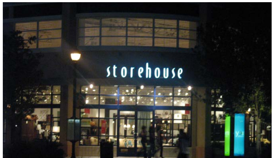
Signage that is internally illuminated is easy to read at night and strengthen the identity of the individual store and overall area. External lighting sources should be focused and low intensity. Additional creative elements can be added that serve during the day and night.
