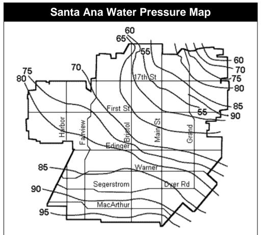
The pressures indicated in this map are approximates. Water pressures fluctuate. It is recommended to check the delivered water pressure to determine if a pressure-reducing valve will be required.
