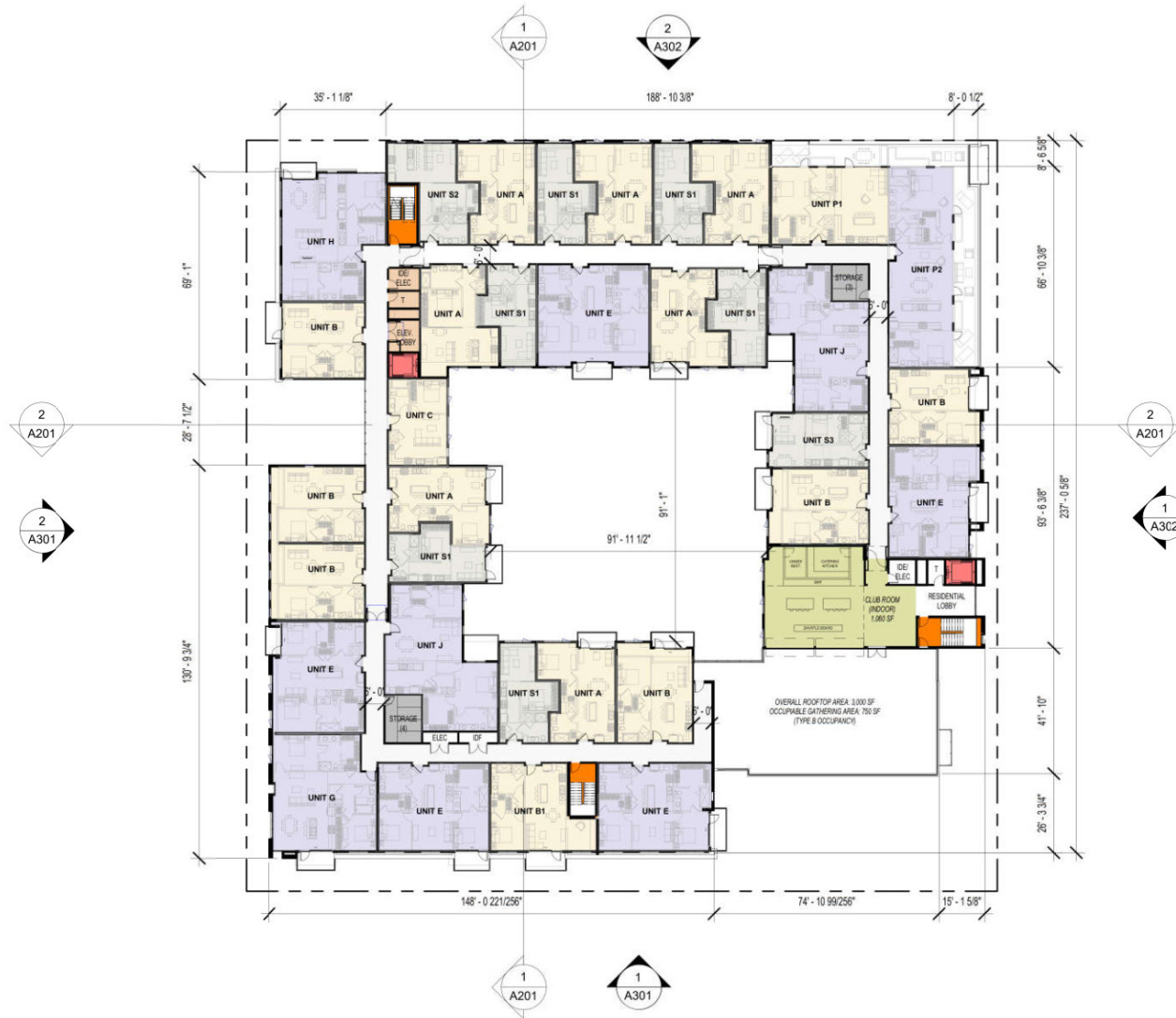
Figure 2-6 Proposed Project Level 7 Residential Unit Design
