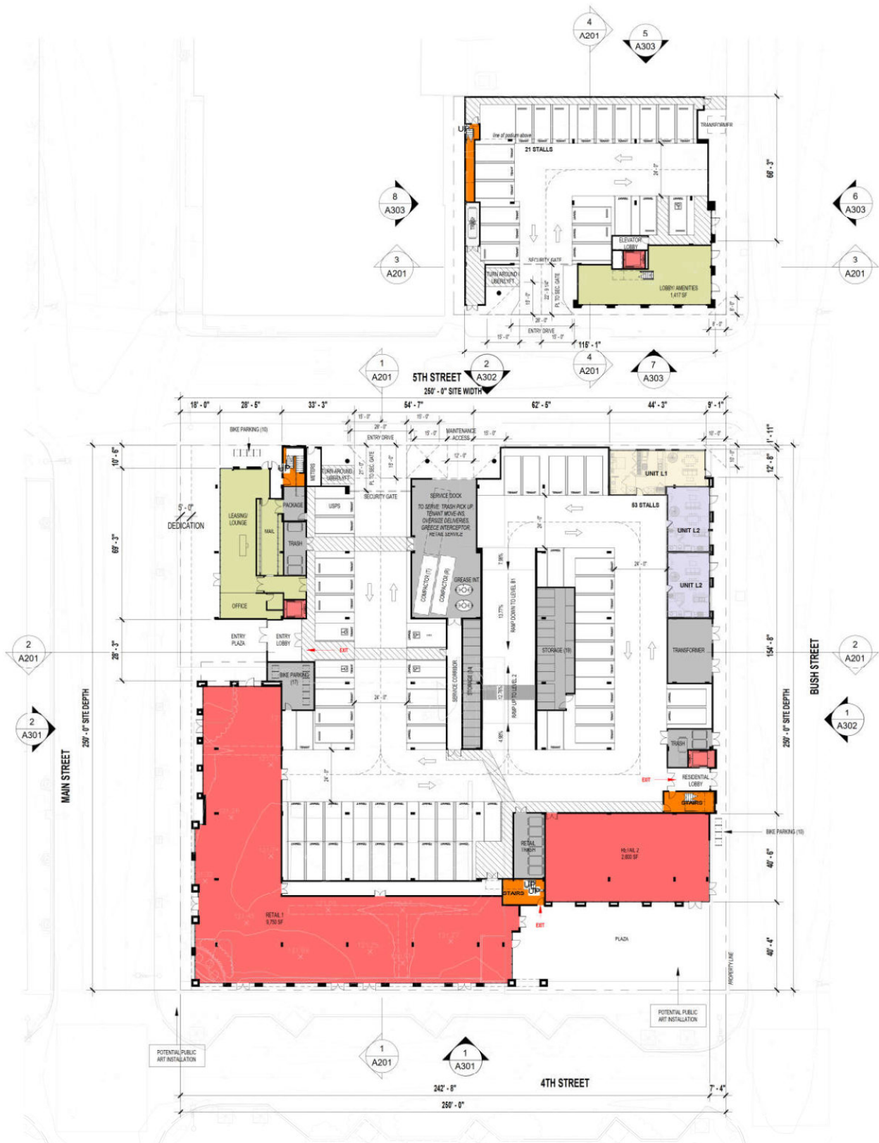
Figure 2-4 Proposed Project Parking Design
