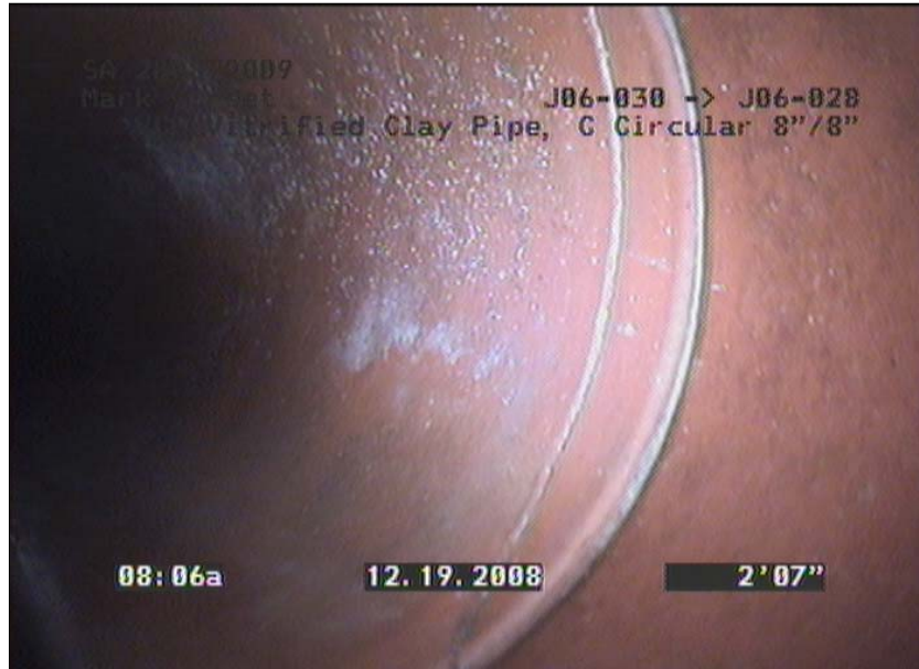
Photo: 27a, Tape/Media No.: 1430, 00:00:00 2.58FT, Fracture Circumferential, from 10 to 01 o'clock, within 8 inch: YES
