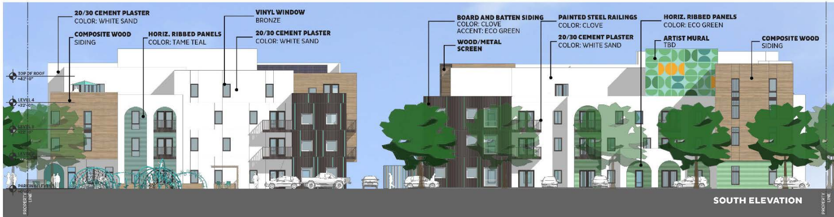
Figure 7 South and East Elevations
