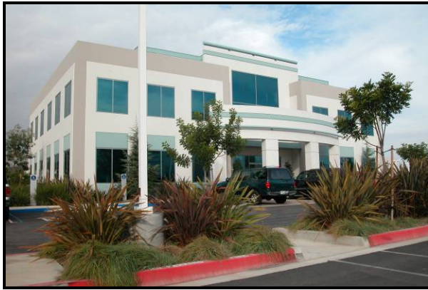
Figure 11-10: Utilize colors, trim to help reduce building scale
