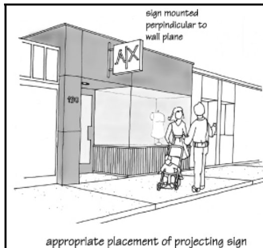
Figure 14-21: Projecting signs should be placed at a 90-degree angle from the face of the building.
