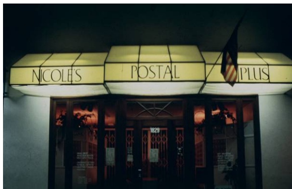
Figure 14-12: Internally illuminated signs should be avoided. Only the sign copy should be illuminated
