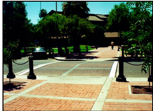
Figure 5-13: This paving visually indicates pedestrian connectivity
