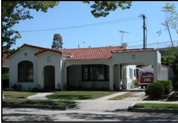
Figure 6-45: Example of porte-cochere
