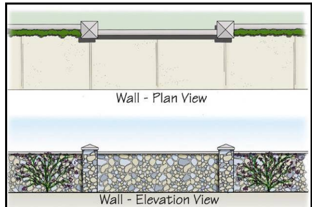
Figure 6-62: Avoid the appearance of long wall planes by incorporated changes in wall planes, pilasters and landscaping
