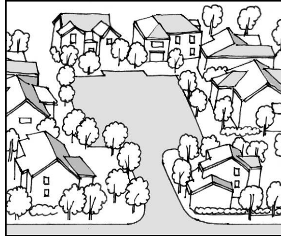
Figure 7-24: Small parking courts with trees that filter views from dwelling units are encouraged
