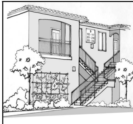
Figure 7-17: Open stairways allow natural surveillance
