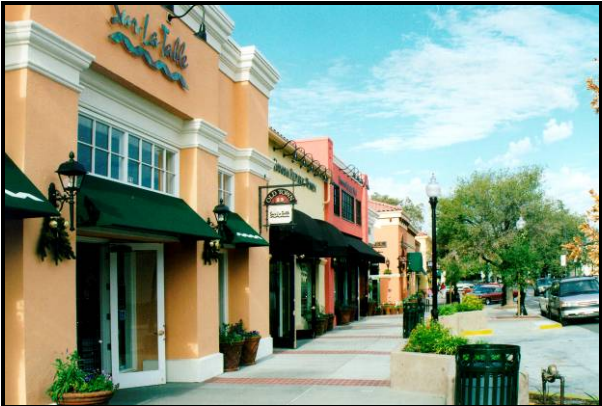
Figure 9-13: Building facade design should incorporate architectural details to reduce scale and mass
