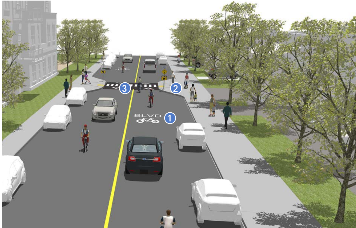
This mid-block design incorporates curb extensions to shorten the crossing distance and provides a level ADA-accessible crossing. This raised speed table also acts as a traffic calming device.
