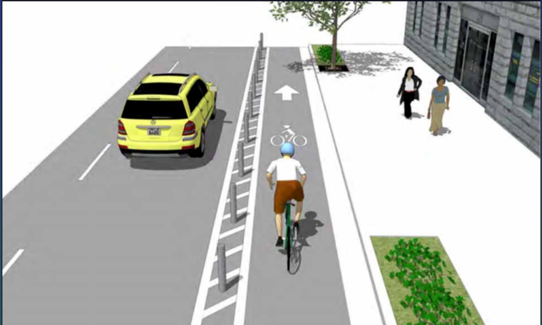
Cycle Track (one-way with bollards)
