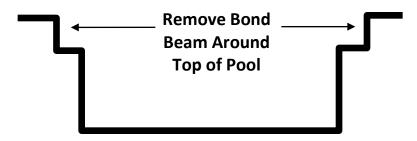
Typical depth of bond beam is 12" - 18"
