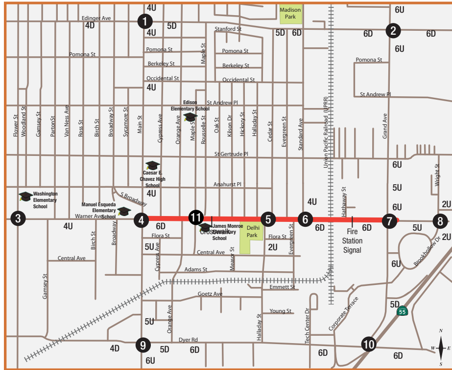
FIGURE 4-1 Roadway and Intersection Geometry With Project
