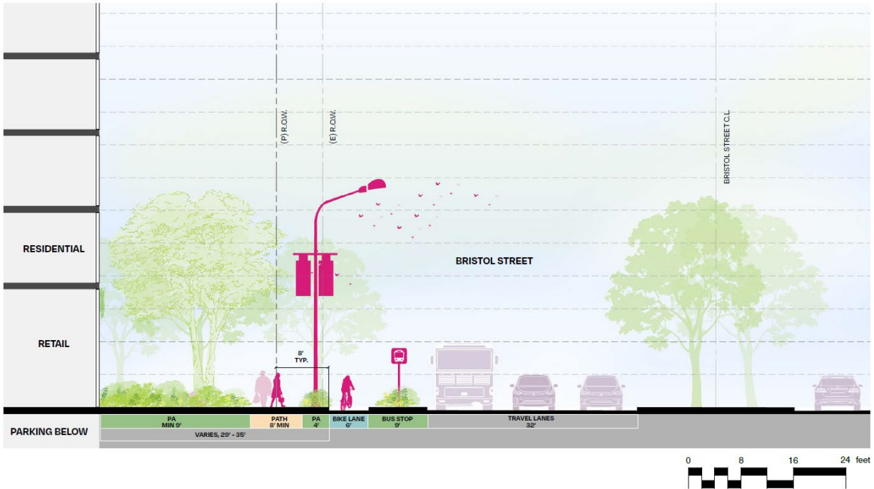
Figure 5-8 Typical Streetscape Section A (Bristol Street)
