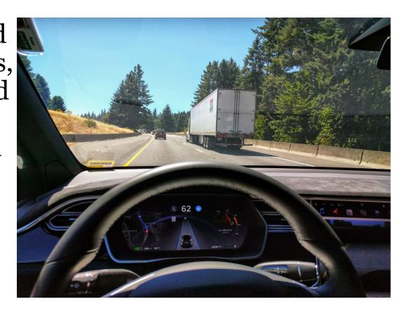
Driver is a necessity, but is not required to monitor the highway environment. The driver must be ready to take control of the vehicle at all times with notice.
