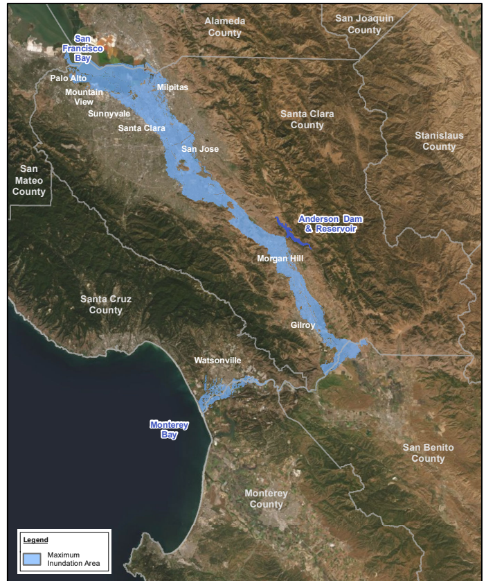
Maximum Flood Area from Anderson Dam Failure
