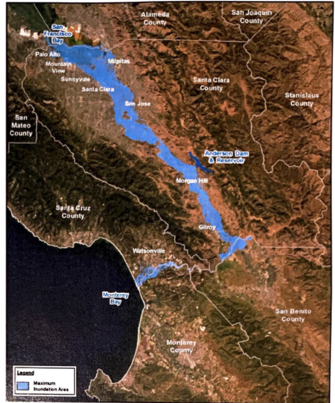
Maximum Flood Area from Anderson Dam Failure
