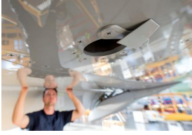
Noise-reducing vortex generators Image Source: Condor
