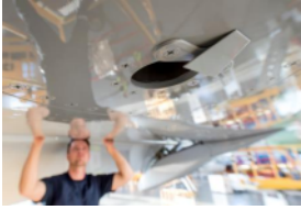
Noise-reducing vortex generators Image Source: Condor
