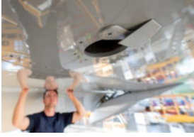
Noise-reducing vortex generators Image Source: Condor
