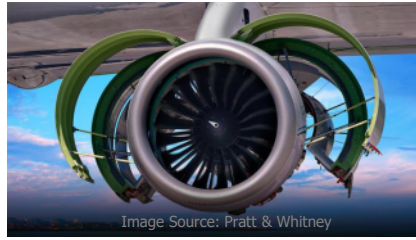
Ultra-high bypass geared turbofan engine
