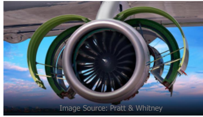
Ultra-high bypass geared turbofan engine
