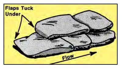
Stagger the joint connections when multiple layers are necessary. For unsupported layers over three (3) courses high, use the pyramid placement method.
