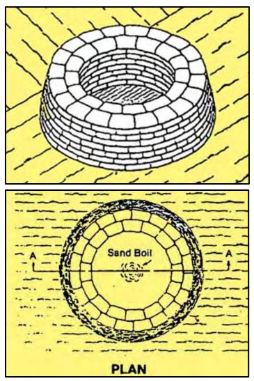
Ring the boil with sandbags, with the first bags back 1-2 feet from the boil. More, if the soil is unstable.
