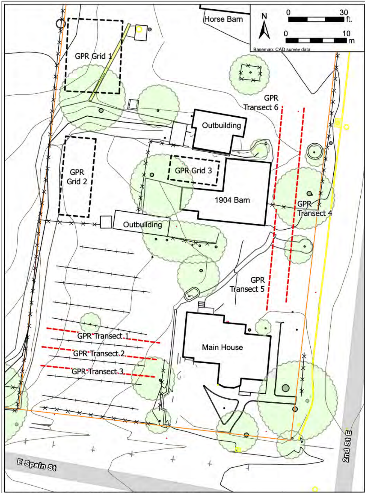
Ground Penetrating Radar Survey Locations 43
