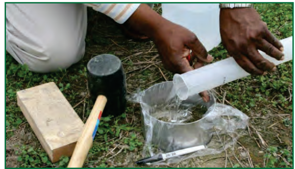
Figure 2.—Water is poured into plastic-lined ring.
