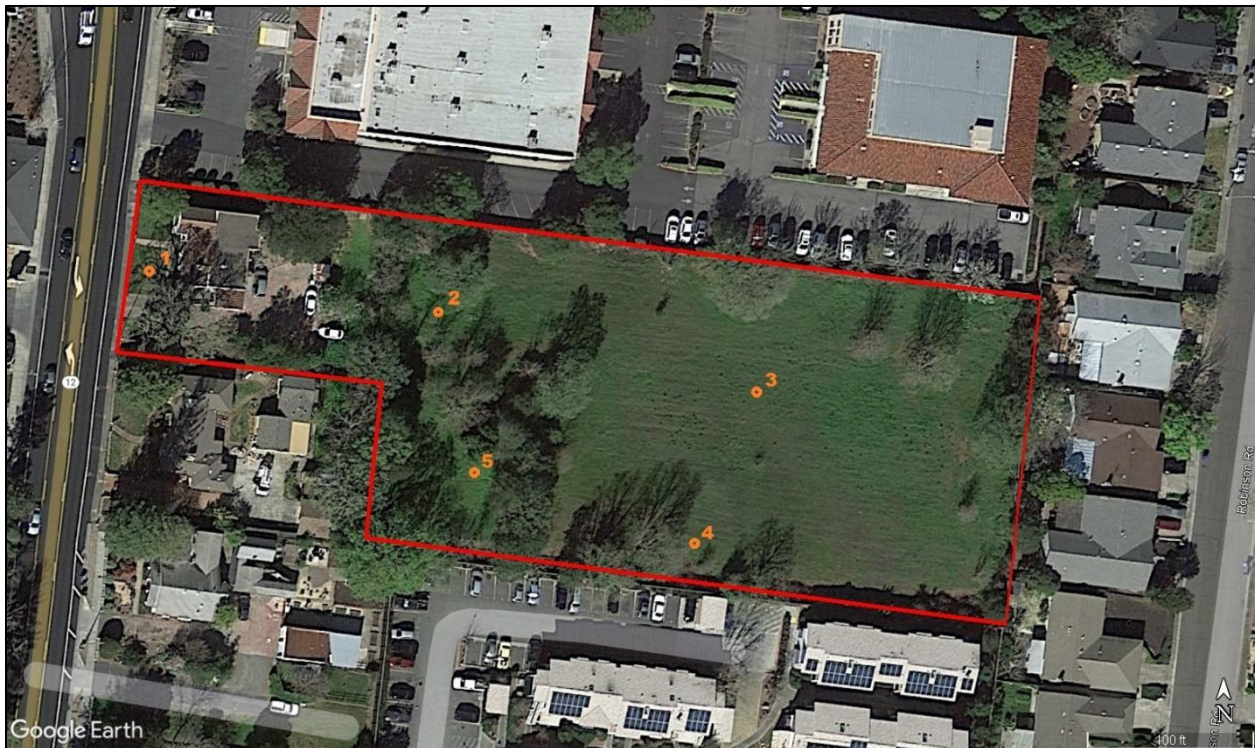
FIGURE 4 -- THE APPROXIMATE AUGER LOCATIONS WITHIN THE PROJECT AREA NUMBERED IN THE ORDER COMPLETED
