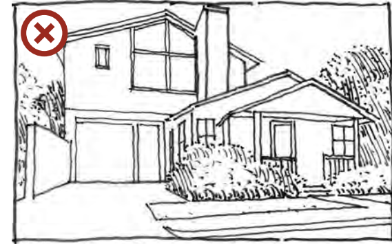
The rear addition is inappropriately large and overwhelms the main building.
