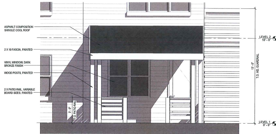
TYPICAL PORCH ELEVATION 10 1/2" = 1'-0"
