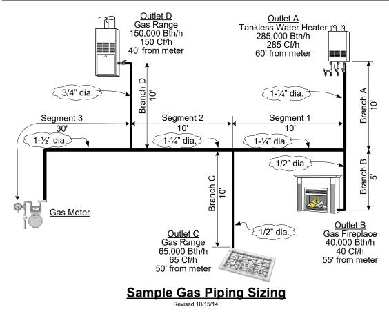
Pipe Size Required 1-1⁄4" dia. 1/2" dia. 1/2" dia. 3/4" dia.
