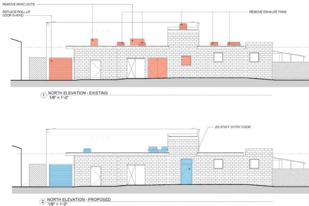
Figure 11. Existing (upper) and proposed (lower) elevation drawings of the subject building's rear, north façade. Elements proposed for removal shaded red, proposed new elements shaded blue. Source: RossDrulisCusenbery Architecture, Inc., 2022, edited by Page & Turnbull
