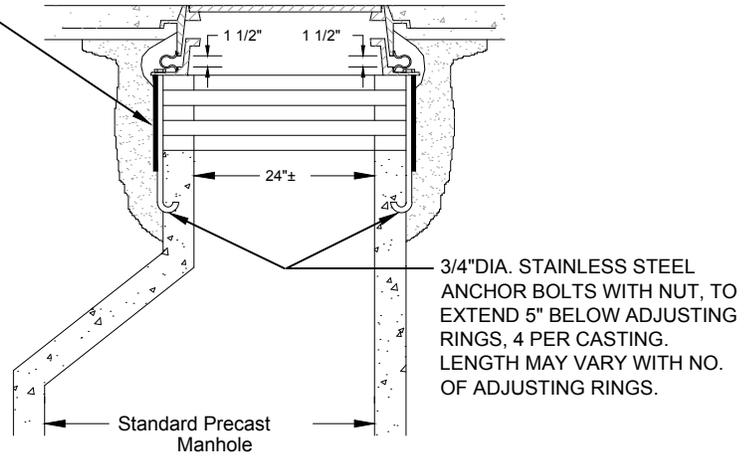
**CROSS SECTION OF CONNECTION TO CONICAL MANHOLE - TYPICAL**
