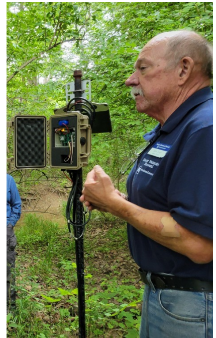
Gary Grahl shows Master Watershed Steward trainees the components of an in stream, real time water quality sensor station in Leesport, PA.
