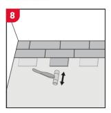
After installing the entire row, use a scrap piece and rubber mallet to gently tap the planks into the previous row to make sure they are tightly locked together and to ensure there are no gaps between the long sides of the planks in any row. Any gapping between planks can result in failure of the entire installation!
