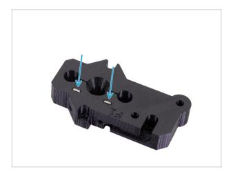
Insert two M3nS nuts all the way down into the MINI-z-top part. Make sure the nuts are fully inserted.
