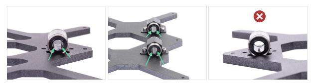
• The correct orientation: When placing bearings onto the Y-carriage, make sure that they are oriented as shown in both pictures. The tracks (rows of balls) have to be on the sides.
