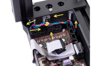
• Connect the Y-axis motor cable to the third slot from the left. Arrange the cable guiding according to the second picture.
