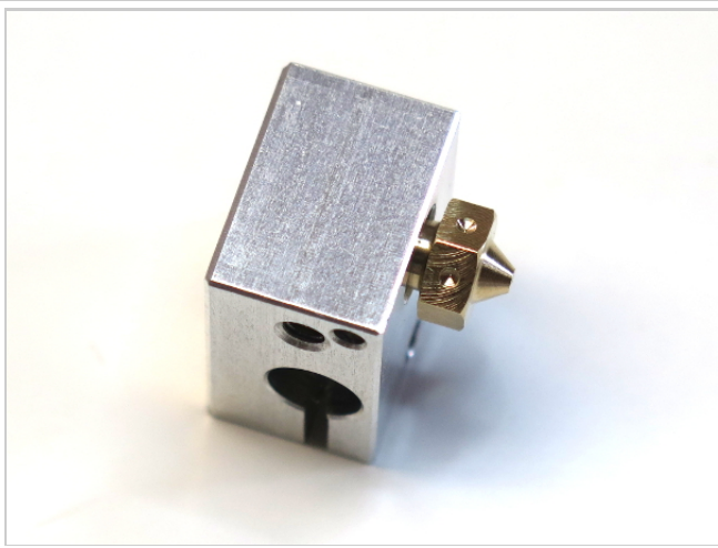
Nozzle screwed into block, and unscrewed a 1/2 turn.
