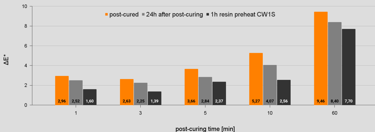
Yellowing \Delta E^* of green body and post-cured sample as a function of post-curing time
