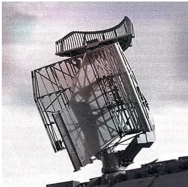
Figure 4-7. IFF antenna above the Target Acquisition Radar
