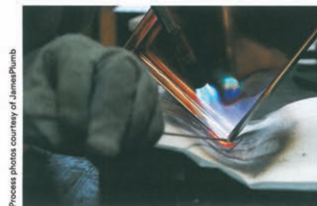
During the brazing process, each corner is heated until it burns cherry-red. Braze is applied and carefully heated until it bonds with the copper.
