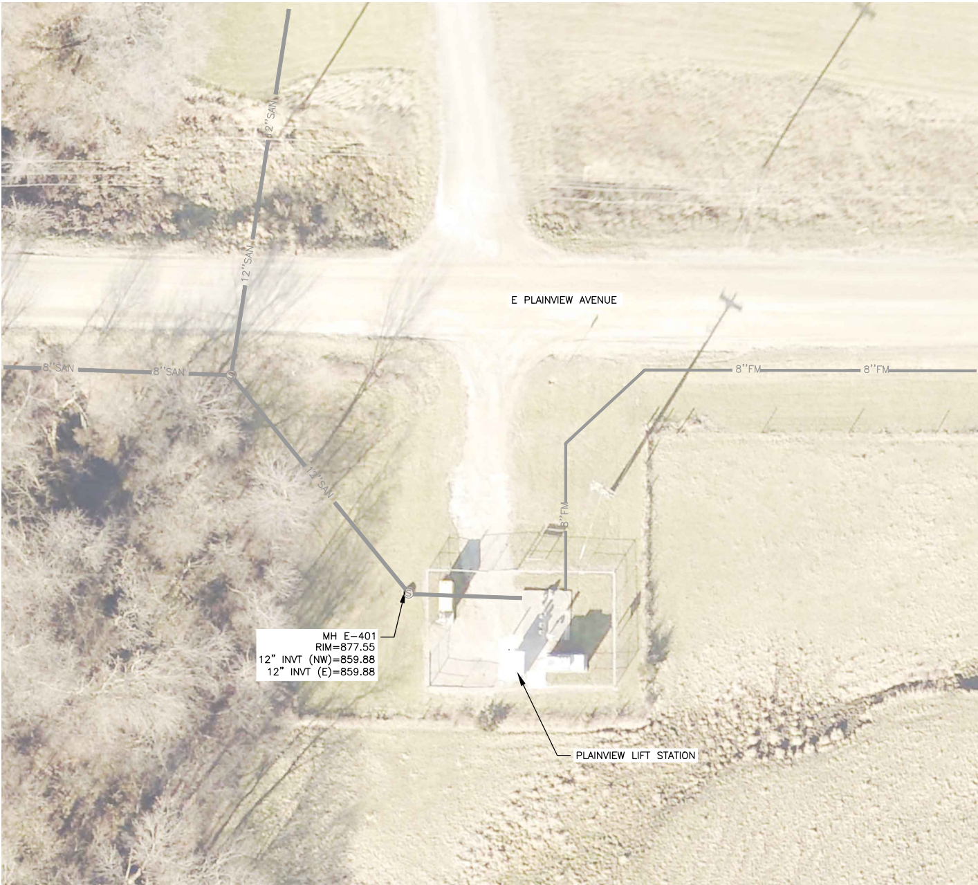
2 Plainview Lift Station SITE LAYOUT SCALE: 1"=20'
