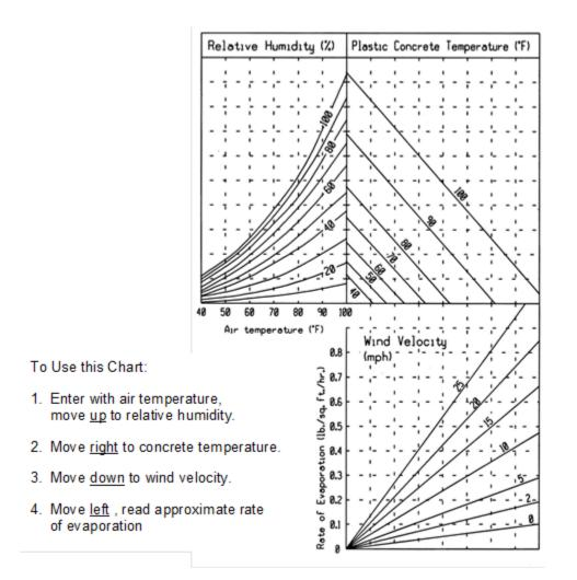
c. If the evaporation rate exceeds 0.1 pounds per square foot per hour but is less than 0.3 pounds per square foot per hour, provide the following concrete evaporation protection.
