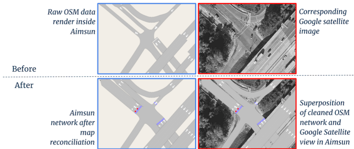
FIGURE 3 Before ( top ) and after ( bottom ) manual editing of the OSM network in Aimsun with comparison to the Google Satellite image.
