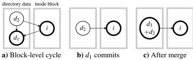
**Figure 4:** Soft-to-hard patch merging. **a)** Soft updates-like dependencies among directory data and an inode block.  $d_1$  deletes a file whose inode is on  $i$ , so Rule 2 requires  $i \rightarrow d_1$ ;  $d_2$  allocates a file whose inode is on  $i$ , so Rule 1 requires  $d_2 \rightarrow i$ . **b)** Writing  $d_1$  removes the cycle. **c)**  $d_3$ , which adds a hard link to  $d_2$ 's file, initiates soft-to-hard merging.
