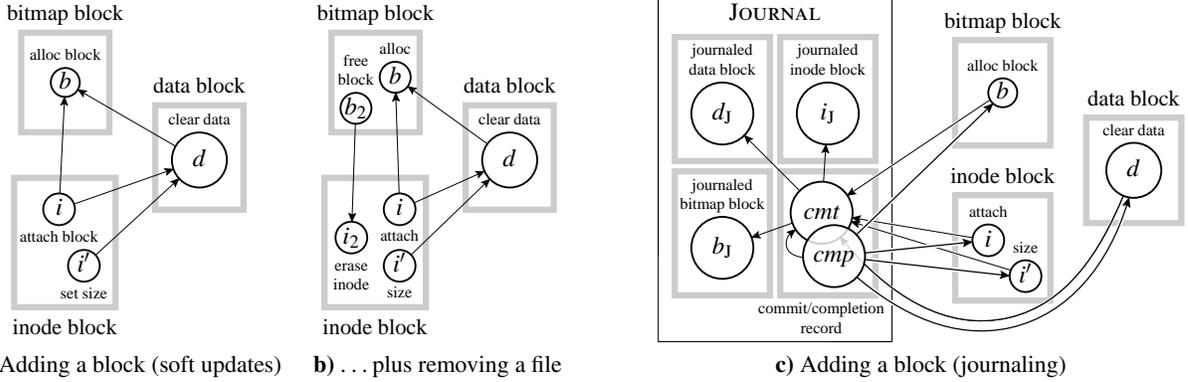
**Figure 2:** Example patch arrangements for an ext2-like file system. Circles represent patches, shaded boxes represent disk blocks, and arrows represent direct dependencies. **a)** A soft updates order for appending a zeroed-out block to a file. **b)** A different file on the same inode block is removed before the previous changes commit, inducing a circular block dependency. **c)** A journal order for appending a zeroed-out block to a file.
