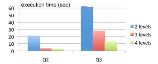
Figure 11: Execution time as a function of serving tree levels for two aggregation queries on  ${\cal T}_2$
