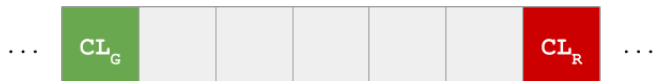
Figure 2: CL_G denotes the version of HEAD when tests were passing. CL_R denotes the version of HEAD when tests are failing. Tests have only been executed at versions CL_G and CL_R , but not in between. Any CL submitted within (CL_G, CL_R] can be the CL that caused the tests to fail, called the culprit CL .
