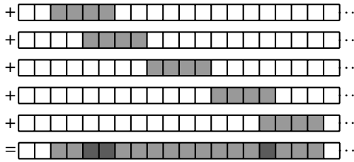
Figure 3. Example Aligned Loop Operation on 17 bytes. Two partially overlapping operations are used at the beginning and at the end. All remaining bytes are handled using aligned non-overlapping Block Operations.
